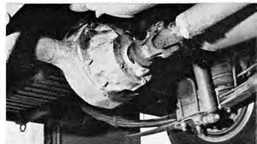
If that rear axle looks on the beefy side, remember that it's one of those elephantine T-Bird jobs. Axles for this honey are super-big 31-spline.
