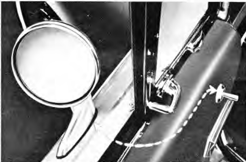
REMOTE CONTROL mirror mounts on driver's door, is controlled by a lever on the inside panel. Both horizontal and vertical movement are controlled mechanically. Diagram below shows how headroom is increased by tilting windshield slightly forward.
