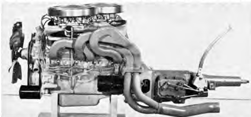
MAXIMUM PERFORMANCE is guaranteed with the Ramcharger 426 engine, Dodge's drag-strip stormer. Modifications announced in June will carry through '64; included are new headers, bigger carburetors, higher-lift camshaft, modified heads, rods and crank.
