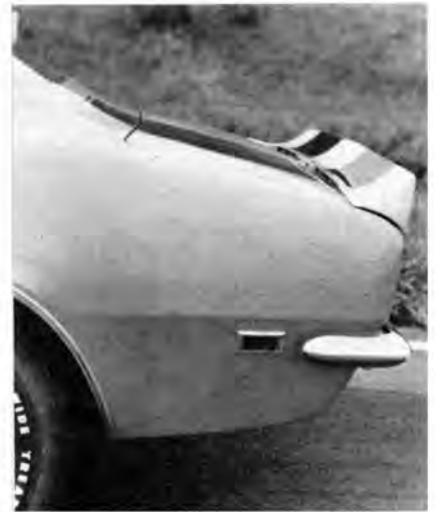
SPOILER on deck lid is appropriate addition to race-oriented Z/28.
