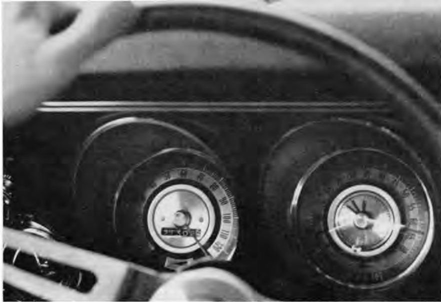
DEEP GEARING is evident in picture of indicated 130 mph speed at 6300 rpm. Great Z/28 engine was still pulling at this speed, and running free and smooth.
