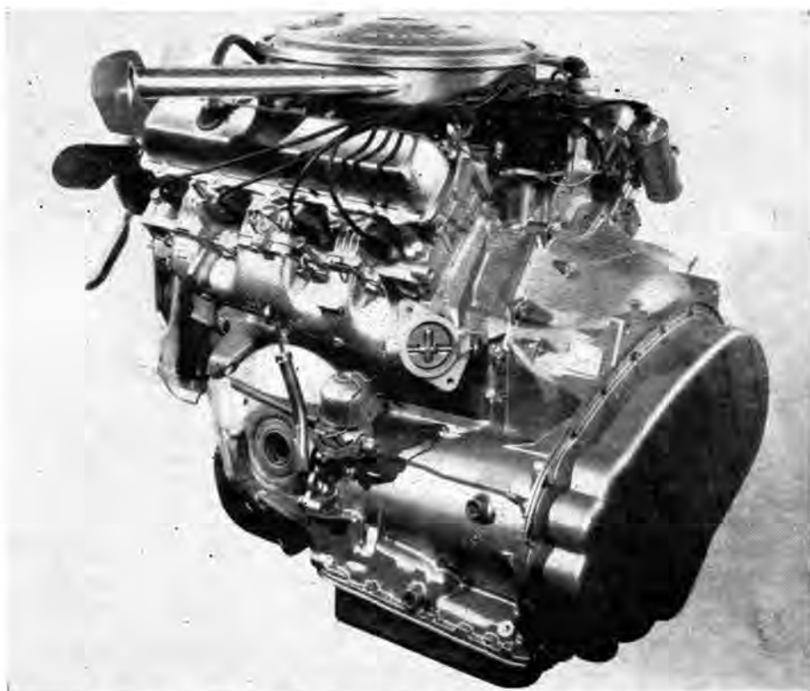
THOUGH THE engine is not new, the transmission arrangement is. This is Oldsmobile Toronado's power package with automatic and differential wrapped around side.
