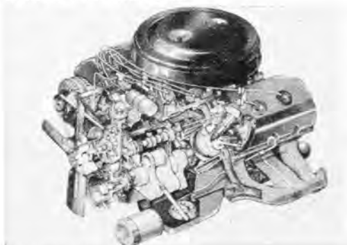
CUTAWAY of Street Hemi shows chamber shape, new manifold.
