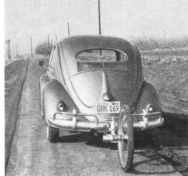
REAR END of the Volkswagen is one of the better views of the bug-like little car, and in this case, one that will be seen quite often. Fifth wheel is for speedometer calibrations, to insure accuracy of test.
