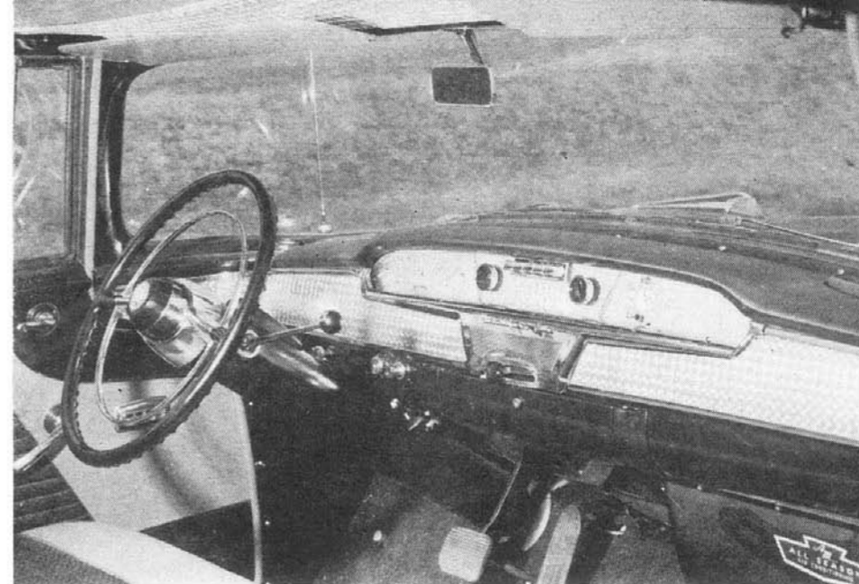
SYMMETRICAL LAYOUT of instrument panel is still favored by Nash Stylists even though it stands alone in this respect. Glove compartment in center of panel, below dash, is augmented by carrier made of netting, running across the car above the windshield. Note air conditioner.
