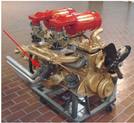
The Hornet also wanted to increase its prowess on the track, and as such, a "7X" special order engine was made available to sponsored racers. In fully prepped form it made about 220 HP and almost 300 ft. lbs of torque!
