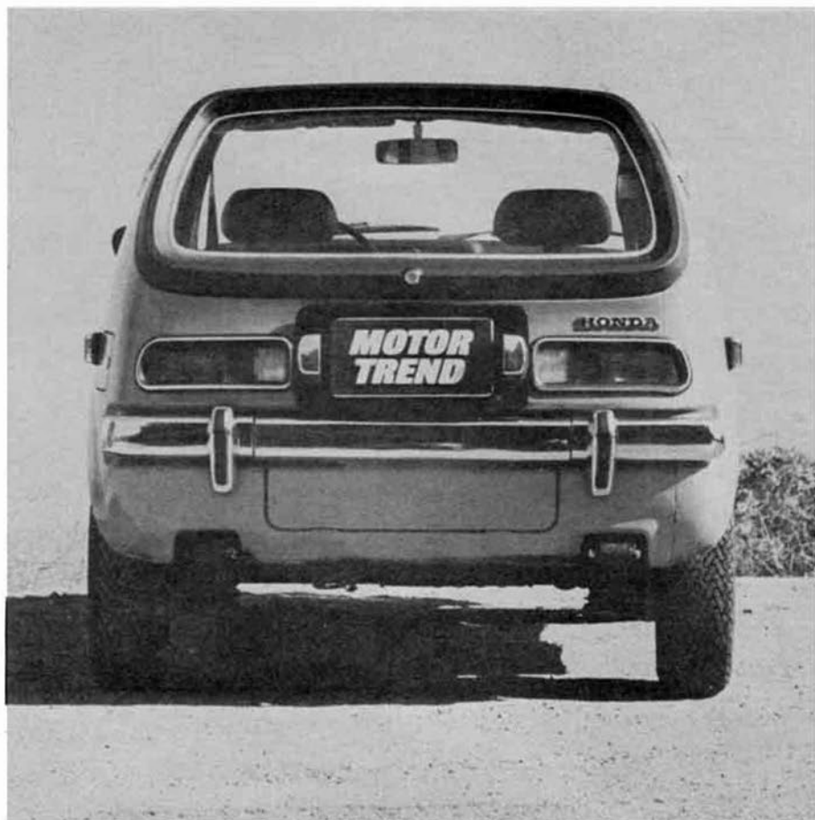
Above: Rear view of Honda makes it easy to visualize interior space-to-exterior size ratio achieved. Locking rear flip-up window simplifies loading of coupe. Below: Honda's all-steel unitized body is surprisingly tight and rattle-free.
