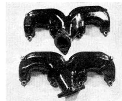
INTAKE MANIFOLDS of aluminum are water jacketed for closer temperature control of fuel-air mixtures that enter the carbs.
