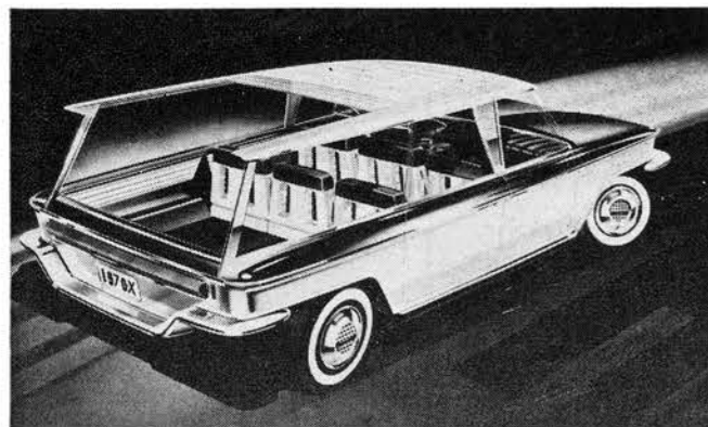
Industrial designer Brooks Stevens, peering into his crystal ball, foresees this "People's Car of Tomorrow" (sometime in the 1970's). Appropriately named "Utopia," the car is powered by a fuel cell—"a cartridge-like replacement for today's motor." A station wagon version features a telescoping roof for fresh air driving or easier loading. The four-door sedan model has luggage compartments
